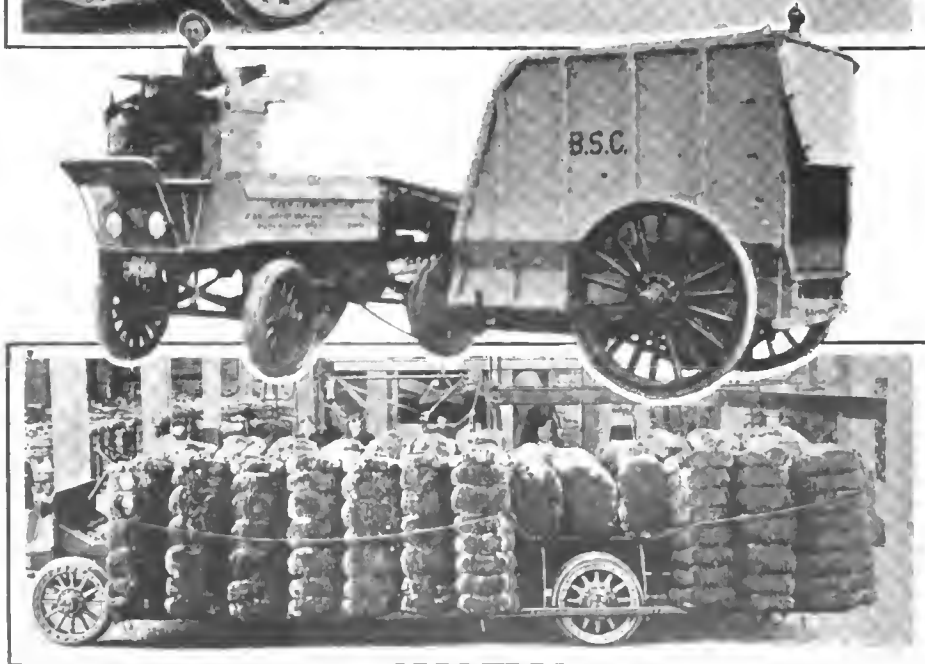
Upper—The modern way of collecting garbage. The low frame allows easy loading Middle—Five-ton electric street cleaning tractor made by the General Vehicle company for use in New York City Lower—Six-ton electric built especially for moving cotton. Loading is facilitated by the underslung frame
